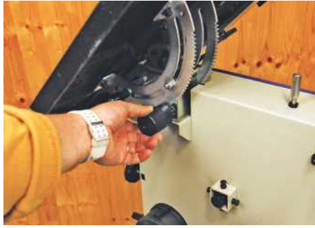
▲ Twin trunions support the table and allow quick angle setting
